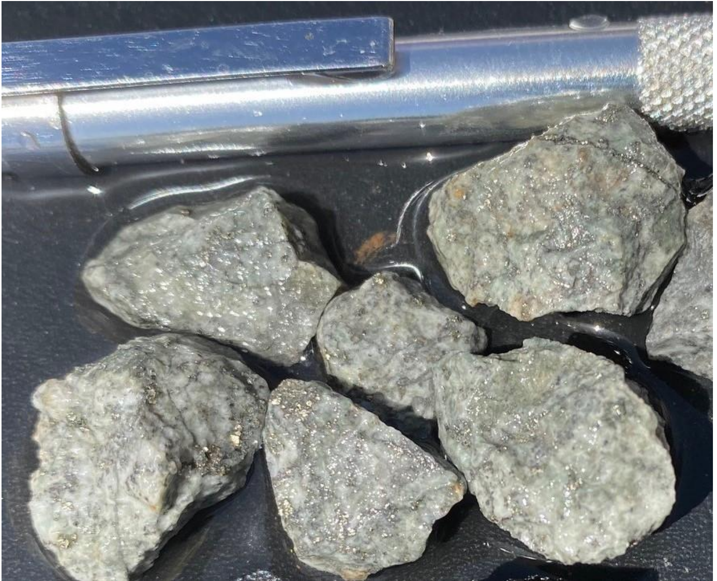
Figure 4 Quartz-sericite-sulphide alteration in RC drill chips (field of view ~10cm)
