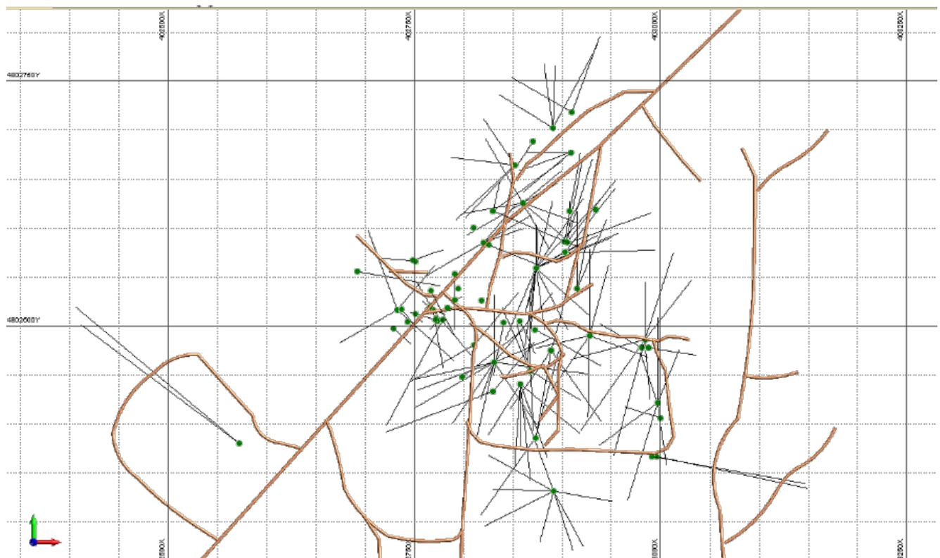
Note: Drill-hole traces are projected to horizontal. Approximate trace of adits is shown in brown. Note that this Novales-Andrea area has been mined in the past and to date no depletion model has been undertaken to identify mineralisation left in-situ.
