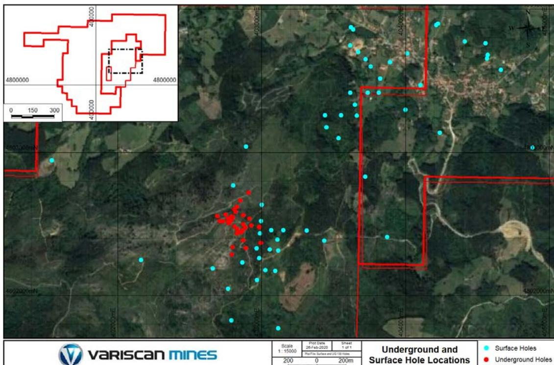
Note: Underground drill-holes shown in red, surface drill-holes in blue. Projected in ETRS89.
