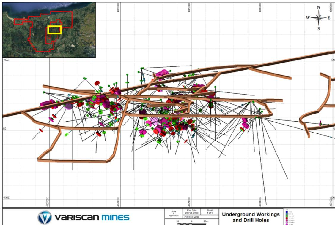
Note: Approximate trace of adits is shown in brown. Note that the Novales-Andrea area has been mined in the past and to date no depletion model has been undertaken to identify mineralisation left in-situ. Drill traces (dip and azimuth) are yet to be verified and may be subject to change.
