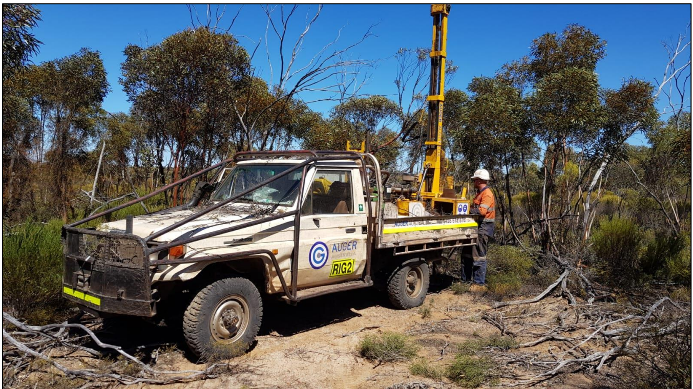
Figure 1. Gyro Australia's Landcruiser mounted auger drill rig will be used to collect low impact geochemical soil samples at CBNP.
