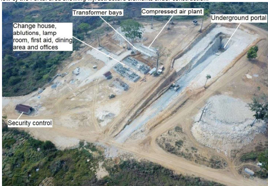
Figure 3: Aerial view of the Portal area showing infrastructure elements under construction.
