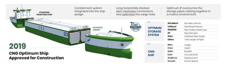
Note: The schematic of the Optimum CNG vessel presented above is indicative of the loading and unloading of CNG using onshore facilities. Modifications to the ship will be made for offshore loading systems such as a STL or SAL system, however it does not require further approvals from ABS for the Optimum CNG containment system.
