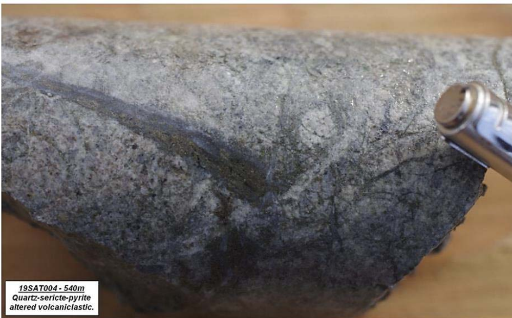
Figure 12 19SAT004 at 540m depth. Quartz-sericite-pyrite veining and alteration overprinting andesitic volcanic rocks.
