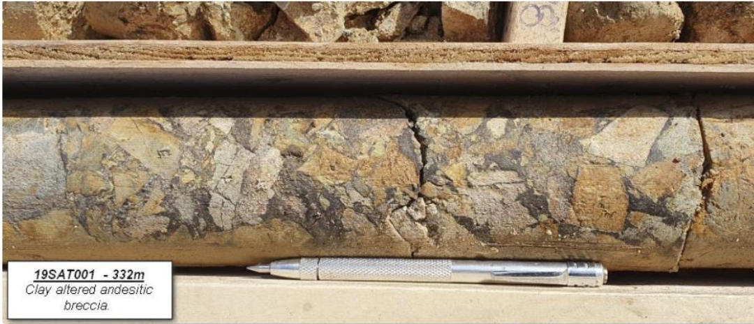
Figure 11 19SAT001 at 332m depth. Argillic alteration overprinting brecciated andesite.
