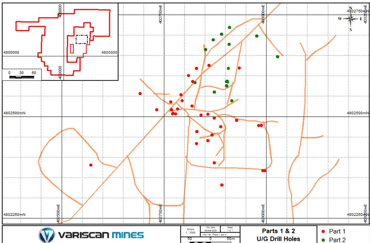
Note: Drill-hole collar locations for 71 historic underground drill-holes (green) and previously announced 130 historic underground drill-holes (red). Approximate trace of adits is shown in brown. Note that this Novales-Andrea area has been mined in the past and to date no depletion model has been undertaken to identify mineralisation left in-situ.
