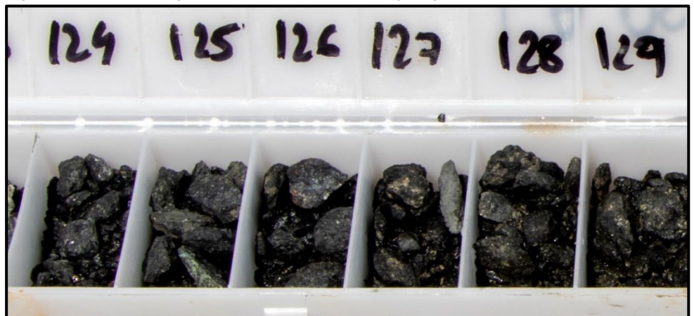
Figure 1 – RC drill chips from LAARC003 showing sulphide rich mineralisation
