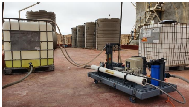
Nano-filtration test rig processing the CE solution at Etango
