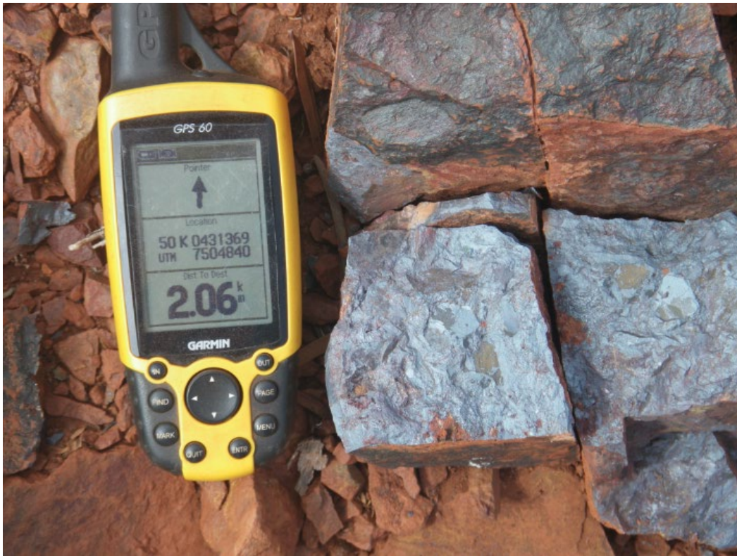
Figure 14: Close up view of hematite conglomerate with hematite matrix as found at Paulsens East
