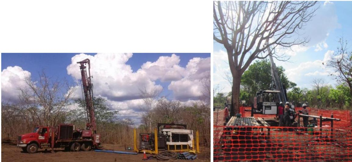
**Figure 5:2 Drilling RC (Left) and DD (Right) at Caula Deposit**
