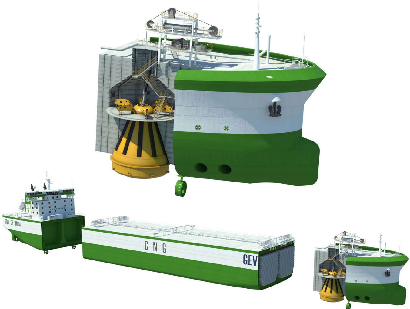
Figure 4: STL equipped CNG Optimum ship with bow and stern thrusters.
