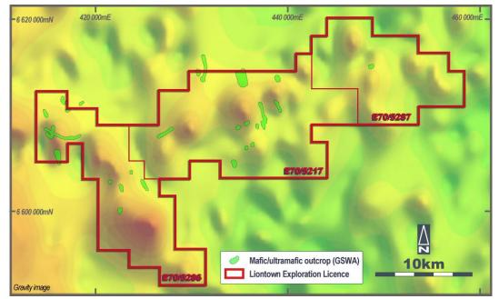
Figure 2: Moora Project: Gravity image (1VD) showing mapped mafic-ultramafic units. (Hot colours indicate dense, possible mafic-ultramafic units).
