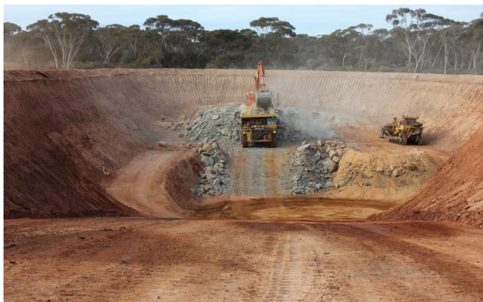
Cassini box-cut following first blasting
