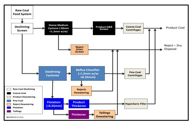
Figure 9: Block flow diagram of the CHPP
