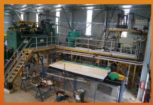
Currently the plant is designed to produce a gravity concentrate and a flotation concentrate that can be cyanided.
