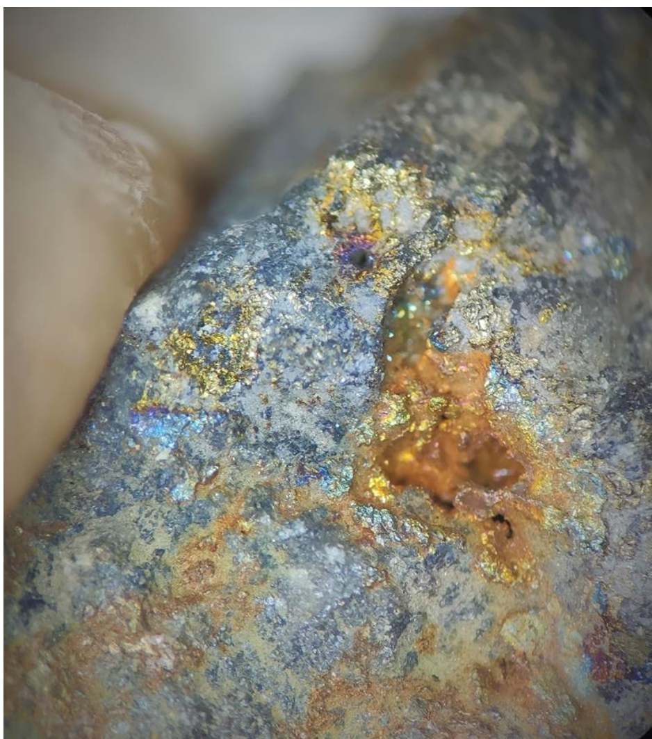
Figure 4. Semi massive sulphides and micro veining within gold mineralised zone at Harris Find. This is more typically associated with a feeder zone related to VMS mineralisation.
