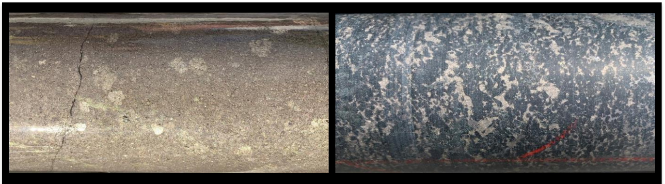
Figure 1. Typical sulphide mineralisation intersected in JD002: hypogene massive sulphides comprising pyrrhotite-pentlandite-chalcocopyrite at ~49.5m downhole ( left ) and matrix/net textured pyrrhotite-pentlandite-chalcocopyrite at ~90.5m downhole ( right ). Core photos of entire zone provided in Appendix 1 .
