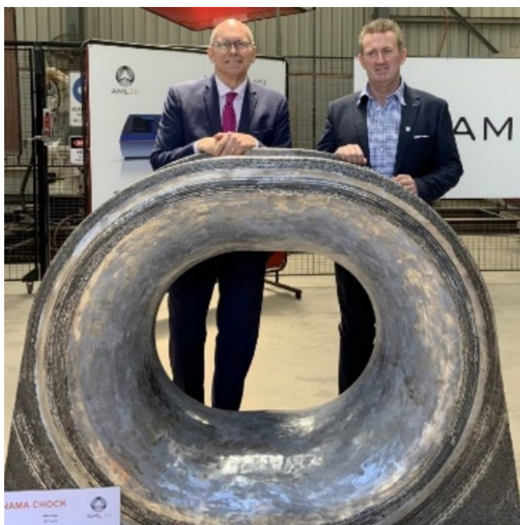
Figure 1 - Panama Chock printed using AML3D's proprietary WAM® process offers more than 1.5 times the strength of a cast version
