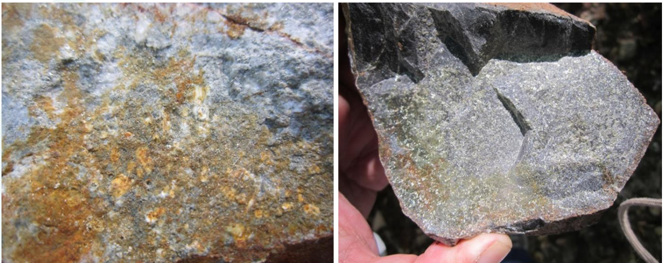
Figure 7 - Disseminated sulphide mineralisation in porphyritic intrusions (left); disseminated sulphide mineralisation in the host rocks (right). Further field evaluations and time will be required to determine average sulphide content, style and individual sulphide constitutions, but to date they have been noted as disseminations and veinlets, with a content range of trace, up to 2% of sulphide mineralisation
