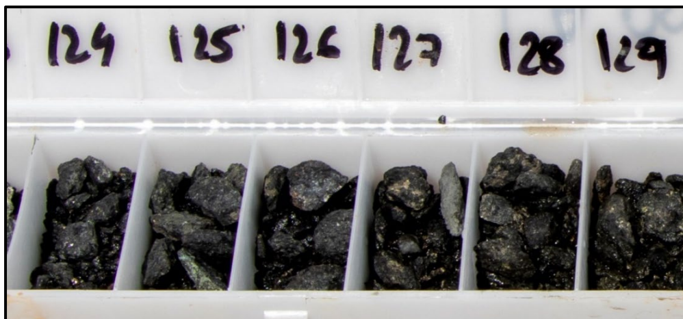
Figure 4: RC drill chips from LAARC003 showing sulphide rich mineralisation
