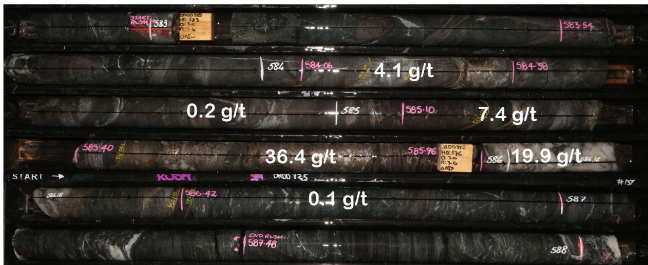
Figure 7: Central Deacon Lode – hole DRDD273, high-grade ore shoot 10% pyrrhotite, trace chalcopyrite and trace visible gold mineralization.
