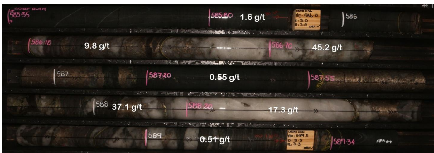
Figure 12: Tribune Lode DRDD360 dominant milky quartz, hosted in moderate biotite/amphibole shearing. Overall 30% sulphide, locally semi-massive with fracture fill to cataclastic textures, chalcopyrite minor with pyrrhotite dominant. Interval assayed 3.2 m @ 9.8 g/t gold.
