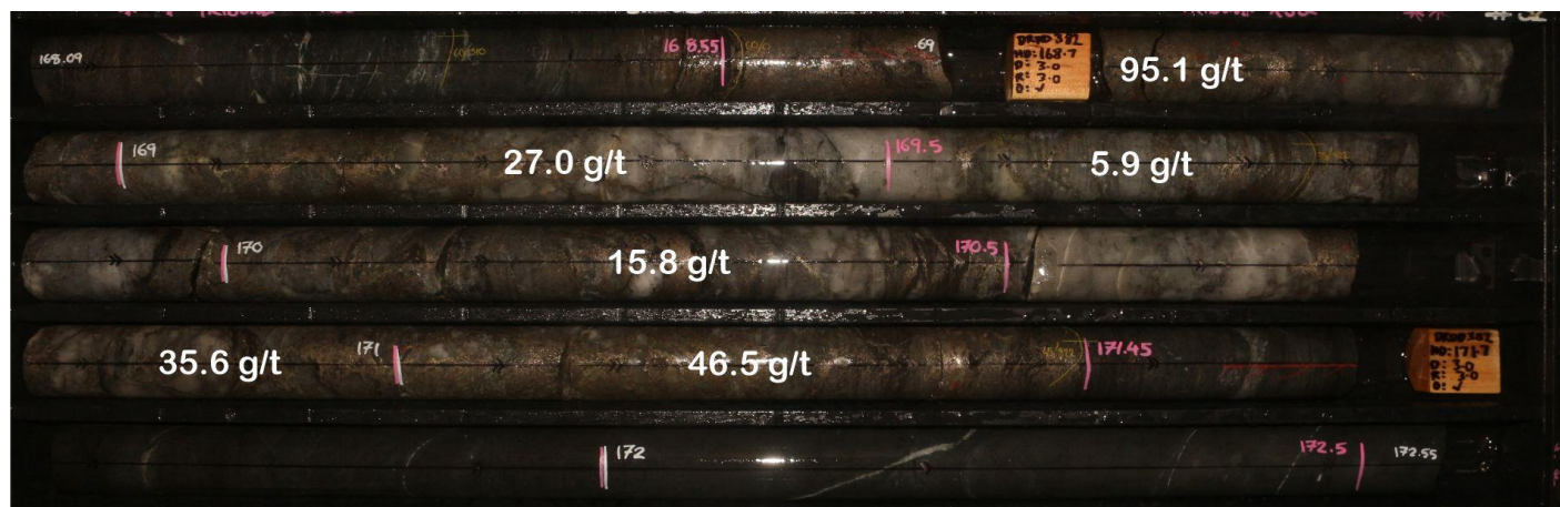
Figure 13: Tribune Lode DRDD382 - Tribune North milky and smokey quartz, hosted in moderate biotite/amphibole shearing. Overall 30% sulphide, locally semi-massive with fracture fill to cataclastic textures, chalcopyrite minor with pyrrhotite dominant +35 flecks of gold logged. Interval assayed 2.9m @ 36.5 g/t gold
