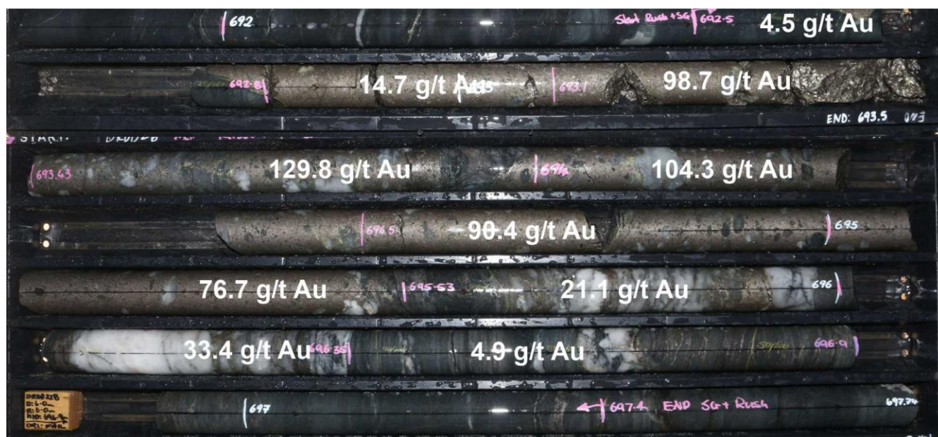
Figure 5: Central Deacon Lode - hole DRDD218 high-grade ore shoot with massive pyrrhotite, trace chalcopyrite, quartz clasts and numerous visible gold grains.
