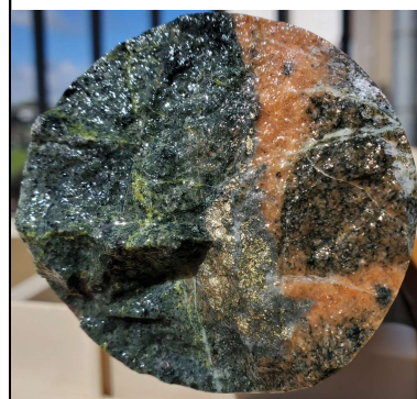
539m – Chalcopyrite veining associated with strongly developed kspar + chlorite (potassic) alteration (interpreted porphyry related)
