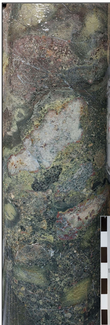
125m - Strongly developed epidote + chlorite + hematite + albite + pyrite (propylitic) alteration (interpreted porphyry related)
