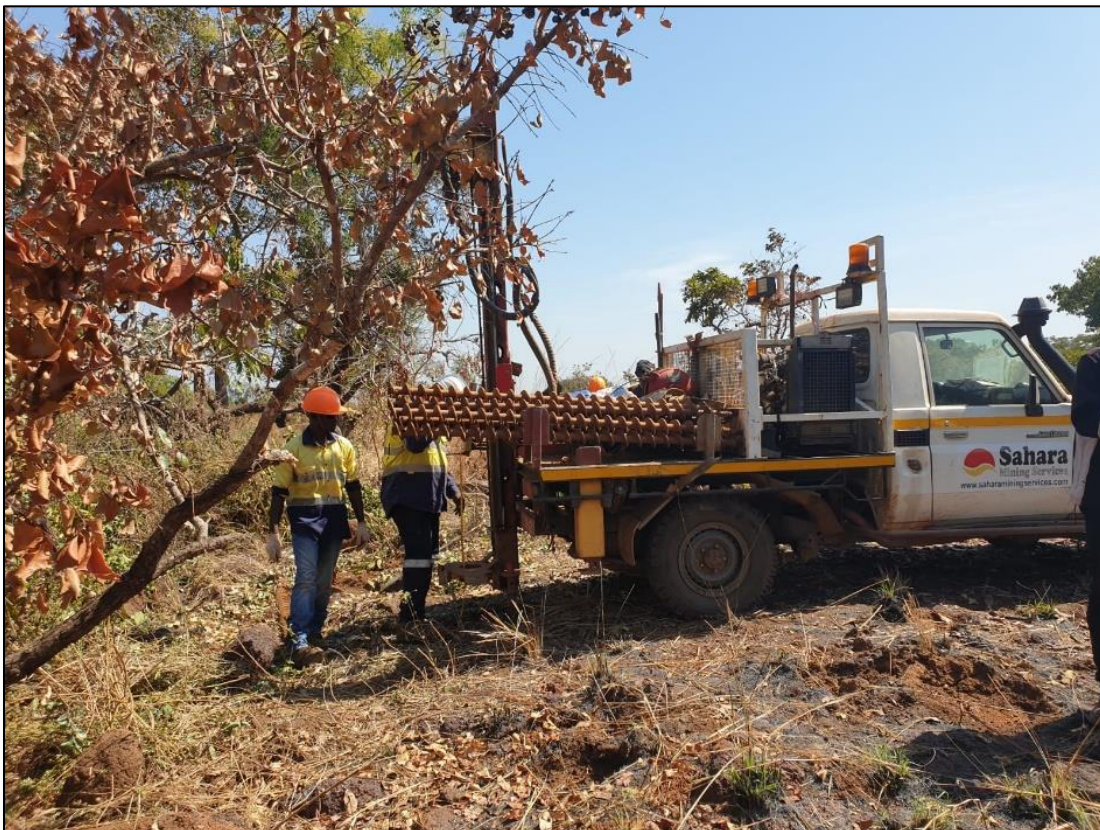
Figure 1 – Power auger drilling on the Kaninko Gold Project, Guinea
