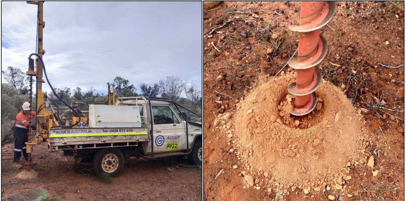
Figure 2. Gyro Australia's Landcruiser mounted auger drill rig collecting low impact geochemical soil samples at CBNP.
