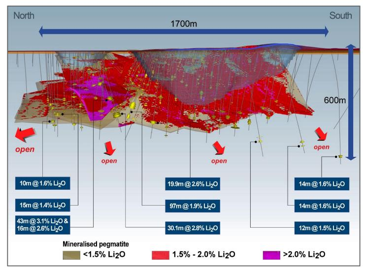
Figure 2: Kathleen Valley – 3D image showing high grade (>1.5% Li<sub>2</sub>O) blocks within block model for interim MRE update, better drill intersections for the Quarter and results recorded at limits of current drilling.
