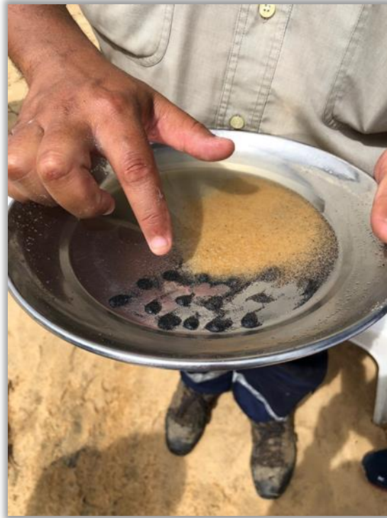
Figure 5 Panning of RC aircore samples from below the water table, during logging at the Mannar Island Project. Dark material is heavy minerals.
