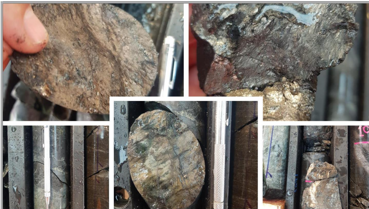
Figure 3: Massive sulphide mineralisation intersected in PLDD006 at approximately 90m depth
