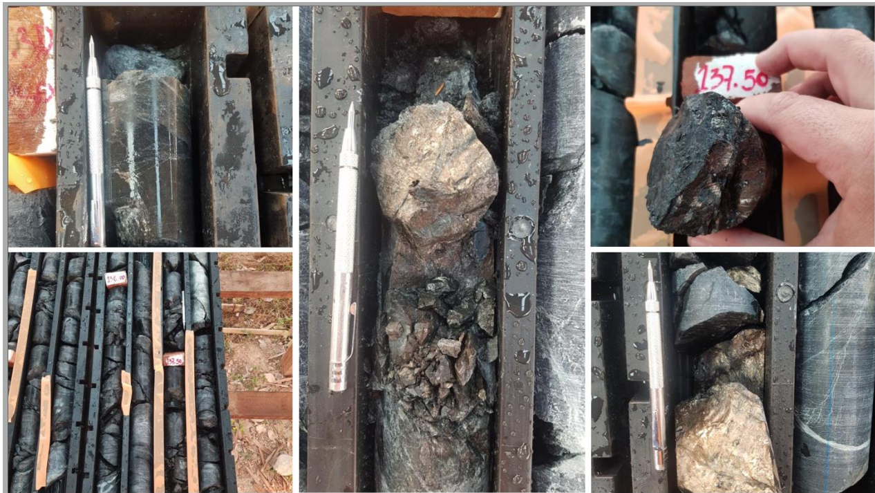
Figure 4: Massive sulphide mineralisation intersected in PLDD008. Orange tape on core trays in bottom left image denotes zones of layered sulphides.
