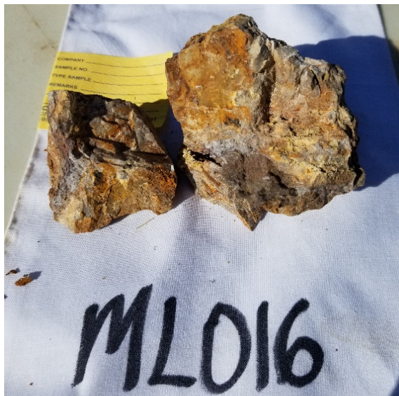
Moccasin Prospect- ML016 Dump sample from small prospecting pit - 4.03 g/t Au, 119 g/t Ag
