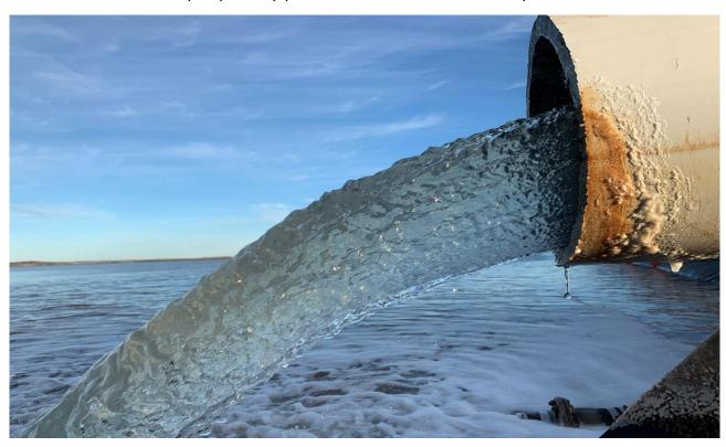
Figure 7: Brine pumped from trench network into Stage 2 ponds
