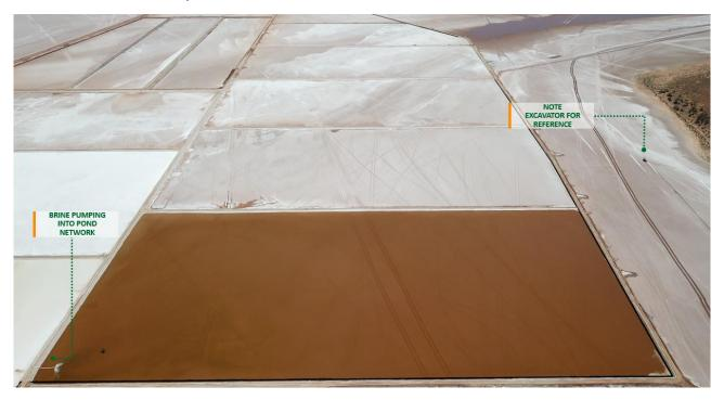
Figure 1: Stage 2 Pond network filling with brine
