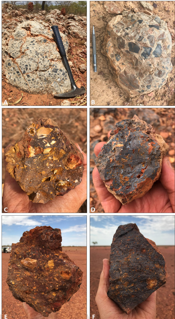
Figure 11 RIGHT: Examples of rock chips from Frewena Far East, including: a) Unsampled silica breccia; b) FFE0006 silica breccia with heterogeneous clasts; c) FFE0011 hematite-goethite-quartz breccia with 0.14% Zn and 148ppm Ni; d) FFE0014 massive vitreous goethite with 0.19% Zn; e) FFE0016 hematite-goethite rich matrix supported breccia with strong limonite overprint, and f) FFE0017 intense hematite-goethite overprinted breccia with pre-existing textures destroyed and reporting 78ppm Co, 89ppm Cu, 108ppm Ni and 483ppm Zn.
