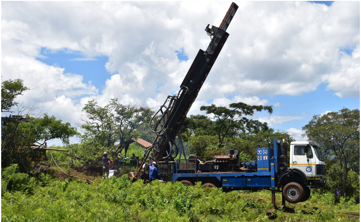
Figure 6: Angled RC drilling testing high grade NdPr rare earth mineralisation associated with vertical carbonatite dykes on the southern margin of the Longonjo Carbonatite, January 2020.
