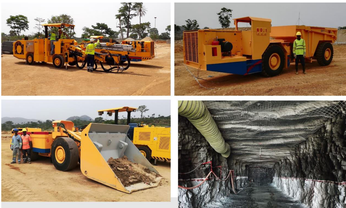
Figure 1: Underground mining equipment and development tunnel with dimensions 6m wide by 4m high.
