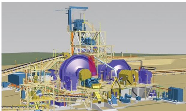
Figure 4: GR Engineering-designed 2.4Mtpa gold process plant
