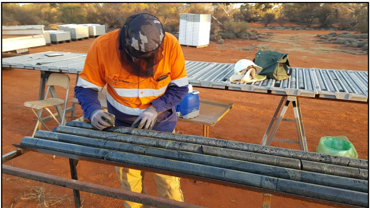
Marking up Massive Sulphides in Diamond Drill Core - RKDD013
