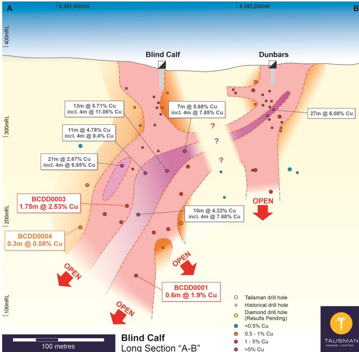
Figure 3: Blind Calf-Dunbars long section showing proposed diamond drill hole targets, current DHEM anomalies and previously reported Talisman and historic drill holes<sup>3</sup>.
