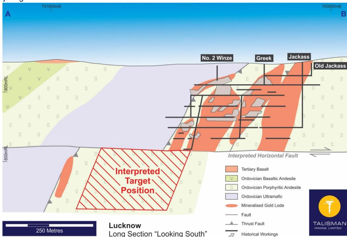
Figure 5: Lucknow Project interpreted long section, showing the interpreted faulted offset mineralisation target position.
