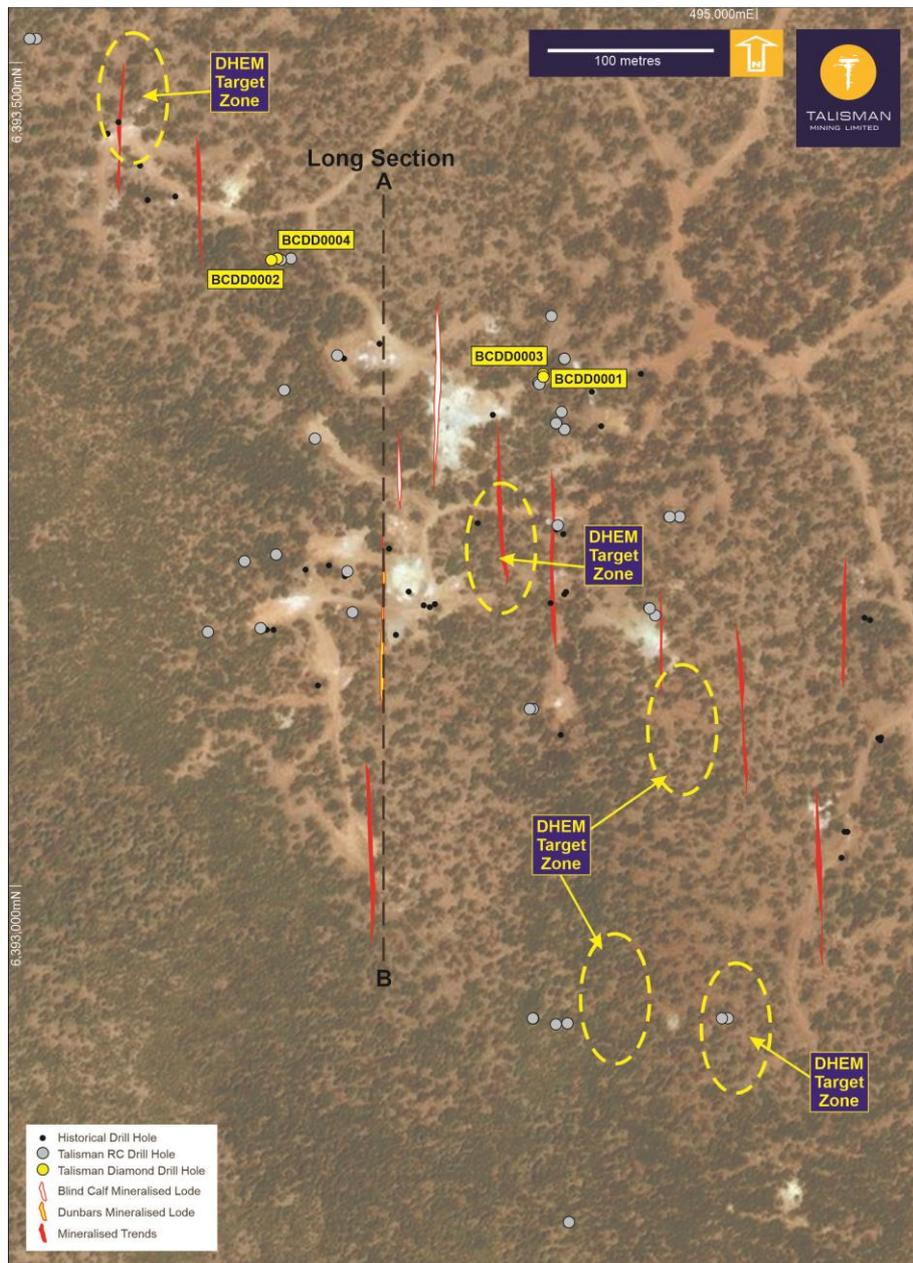
Figure 2: Blind Calf-Dunbars drill collar plan showing position of the completed diamond drill holes, the Long Section positions and the DHEM target zones for future RC drilling
