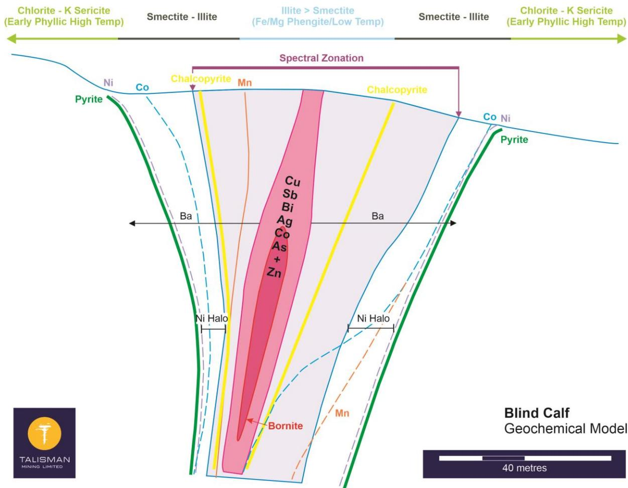
Figure 4: Schematic cross sections illustrating metal and alteration zonation interpreted from Blind Calf RC and diamond drill data
