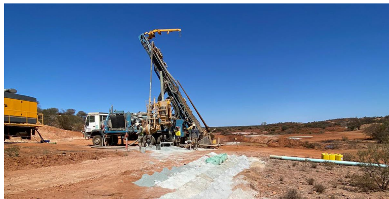
Plate 1 RC drilling underway at Apollo Hill Hanging-walls.
