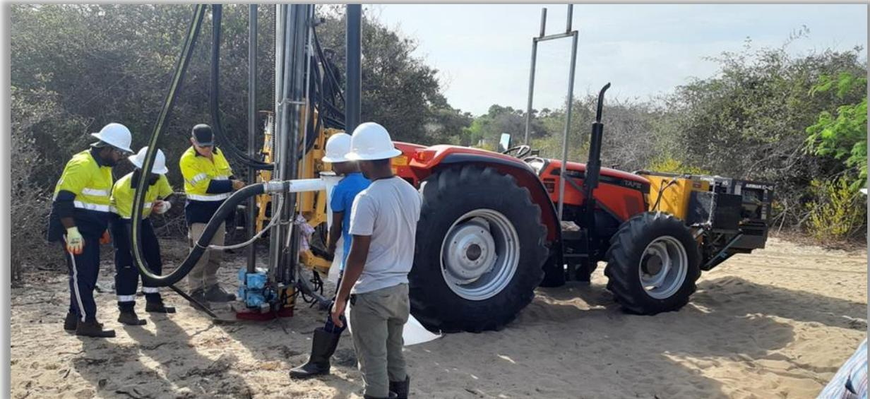
**Figure 4 Titanium Sands Ltd.’s RC aircore drilling rig, training of local crew at Mannar Island.**
