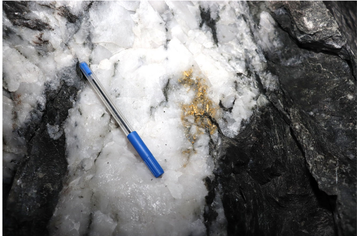
Visible gold exposed in the 2120 ore development drive
