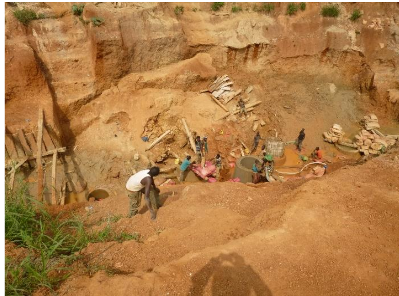
Steel reinforced concrete wells used at Gamina South on 15/12/2014 (Northern end of Abujar Middle tenement)
