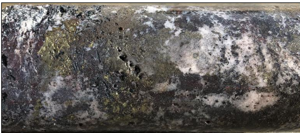
Photo 2. Patchy and disseminated chalcopyrite and pyrite in hematite-quartz veined Cayley Lode mineralisation, SMD086 - 319.9m.
