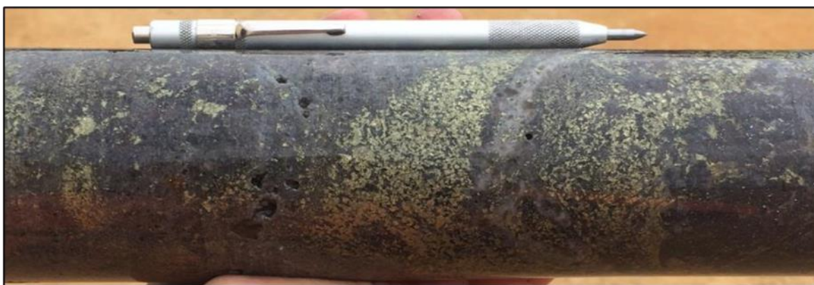
Photo 1. Quartz-chalcopyrite-magnetite-hematite-pyrite mineralised Cayley Lode, SMD085 - 358.8m
