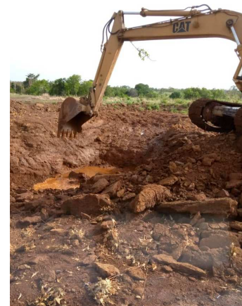
Laterite iron ore pre-strip after blasting and heavy rains.
