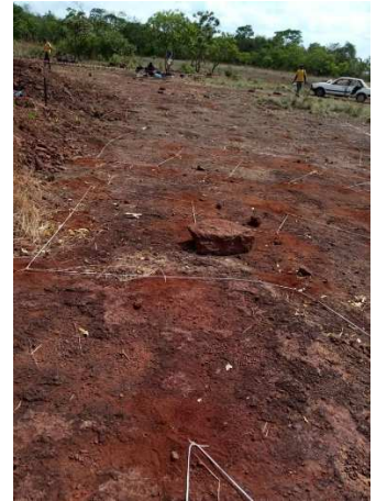
Drilled & Marked Blast Holes Charged & Wired Blast Holes For initial breaking of ~1m surface laterite hard-cap iron ore (lower grade iron ore +/- overburden)
