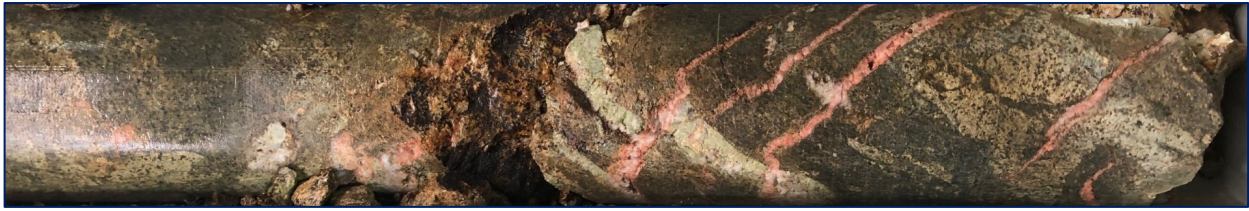
Figure 5: Example of potassic veins, alteration and boxworks after sulphide (H8DD023, 80.5m, NQ core).
