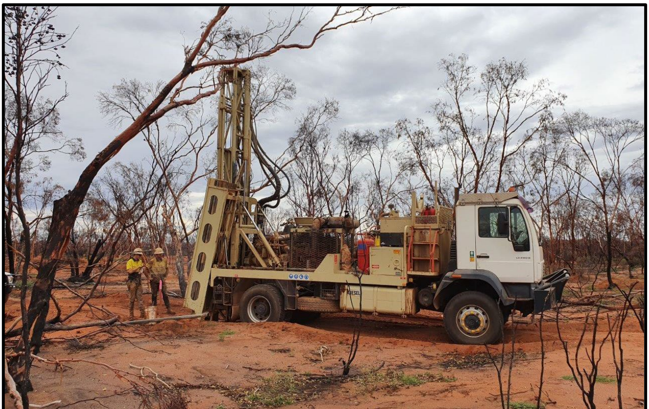
Figure 2 – Reconnaissance Aircore Drilling at the Think Big Prospect in the Fraser Range
