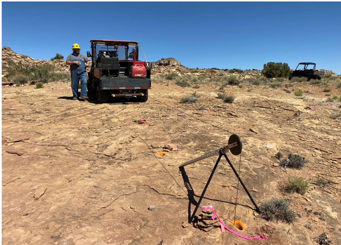
Figure 3: Downhole gamma logging being conducted at the Jeffrey uranium/vanadium project in Utah.
