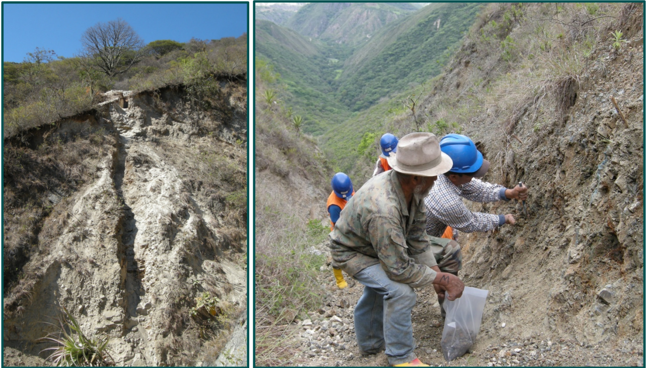
Figure 6 | Lumapamba Prospect, hand-dug trenching across zone of mapped calcite breccia hosting mineralised porphyry clasts. Figure 7 | Representative chip-channel sampling at the Lumapamba gold-copper porphyry target area.
