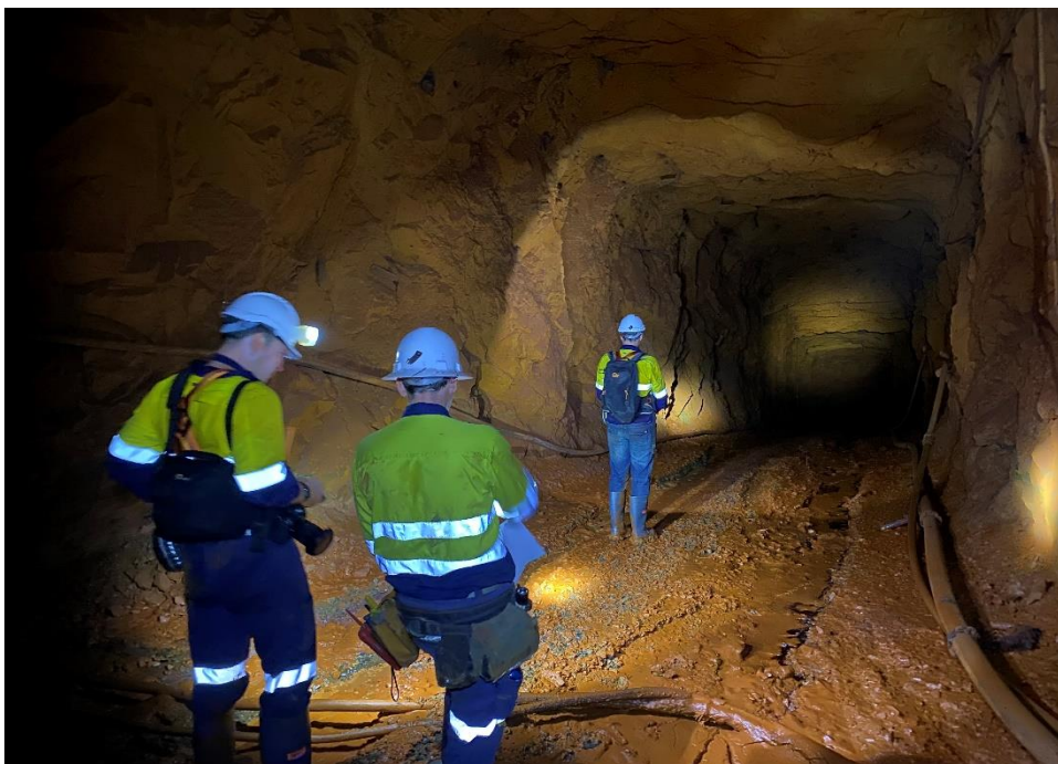
Figure 1: Bellevue technical staff inspecting the recently exposed main decline at the Bellevue underground mine during dewatering activities.
