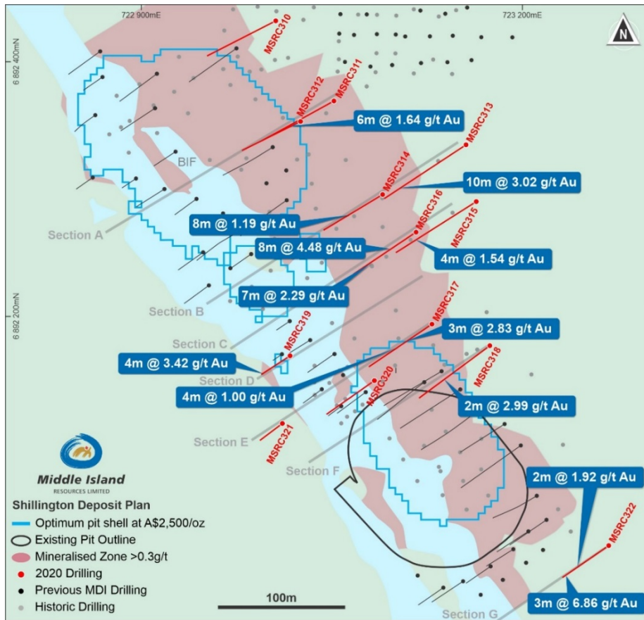
Figure 2 Plan view of the Shillington gold deposits showing new RC drilling results
