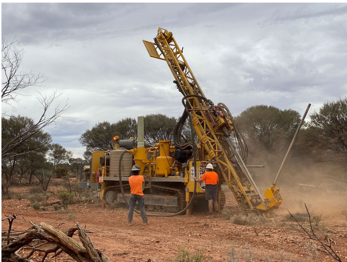
The AC drilling was conducted by HARMEC Pty Ltd using this Edson 3000W track-mounted drill rig. This rig will be converted to a reverse circulation (RC) configuration for follow-up drilling of the new 800 metre gold anomaly.
