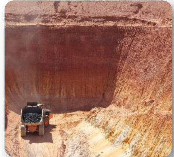
Test pits – 2017 Assessed the digability of overburden and mined 100t of uranium ore
